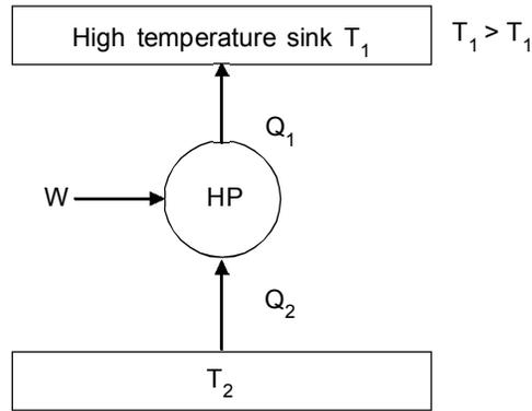
The efficiency of a heat pump cycle is usually called the coefficient of performance. It is the desired effect upon the external work supplied for obtaining that desired effect.
