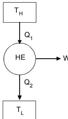
$$\text{Effect} = \frac{\text{output}}{\text{input}} = \frac{W}{Q_1}$$
