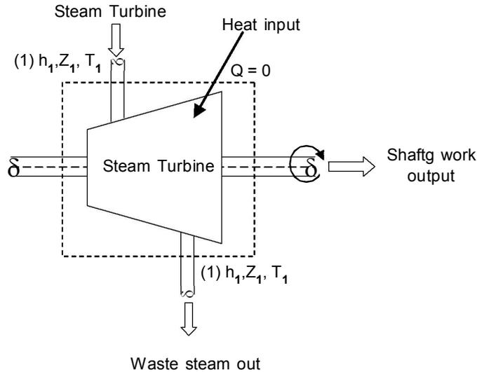
A steam turbine receives a superheated, high pressure steam that experiences its. Enthalpy drop as the steam passes over the turbine blades. This enthalpy drop is converted into the kinetic energy of rotation of the blades mounted on the turbine drum. The turbine is well insulated which gives rise to the maximum work output. The turbine is well insulated.
