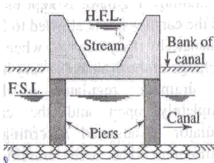
The hydraulic structure in which the drainage is passing over the irrigation canal is known as super passage. It is reverse of an aqueduct. A super passage is similar to an aqueduct, except in this case the drain is over the canal.
