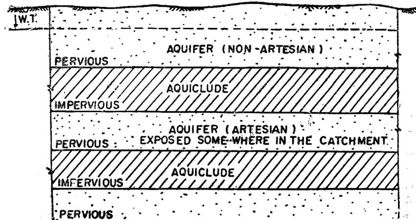
The yield of a well depends on many factors, some of which, such as well diameter, are inherent in the well itself. But all other things being equal, the permeability and the thickness of the aquifer are the most important.
