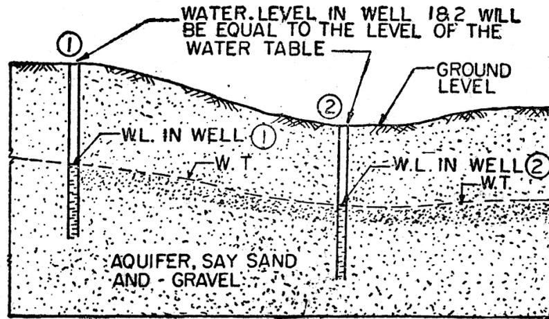
The ordinary gravity wells of 2 to 5 m diameter, which are constructed to tap water from the top most water bearing strata, i.e., from the unconfined aquifers, are known as unconfined or non-artesian wells. The water levels in these wells will be equal to the level of the watertable. Such well are, therefore, also known as wells or gravity wells.
