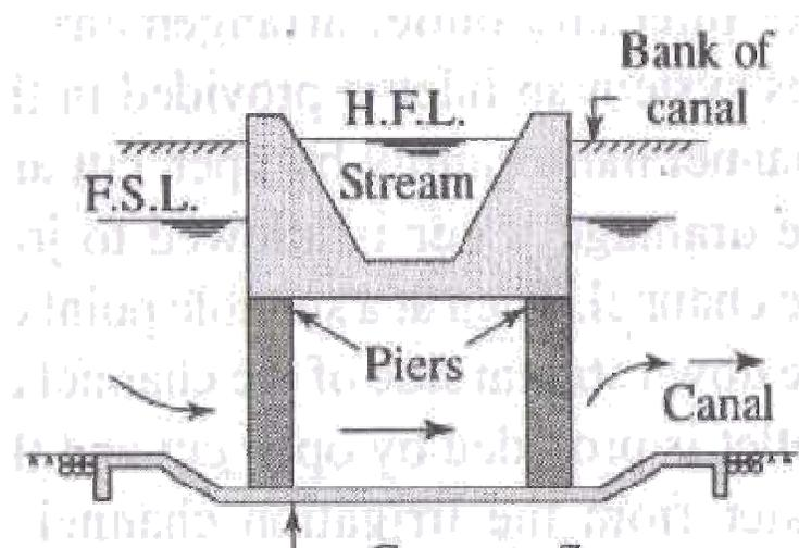
If the FSL of the canal is sufficiently above the bed level of the drainage trough, so that the canal flows under syphonic action under the trough, the structure is known as canal syphon or a siphon super passage.
