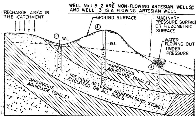
The rains falling in the catchments (i.e., by discharge). However, the water will not rise to this full height, because the friction of the water moving through the aquifer uses up some of the energy.
