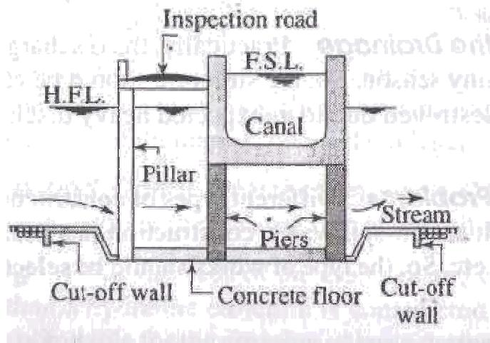
In case of the siphon aqueduct, the HFL of the drain is much higher above the canal bed, and water runs under syphonic action through the aqueduct barrels or tunnels. Here the sloping apron provided on both sides of the crossing. The apron may be constructed by cement concert or stone pitching. The section of the drainage below the canal trough is constructed with P.C.C. in the form of tunnel or barrels. This tunnel acts as a syphon. Cut-off
