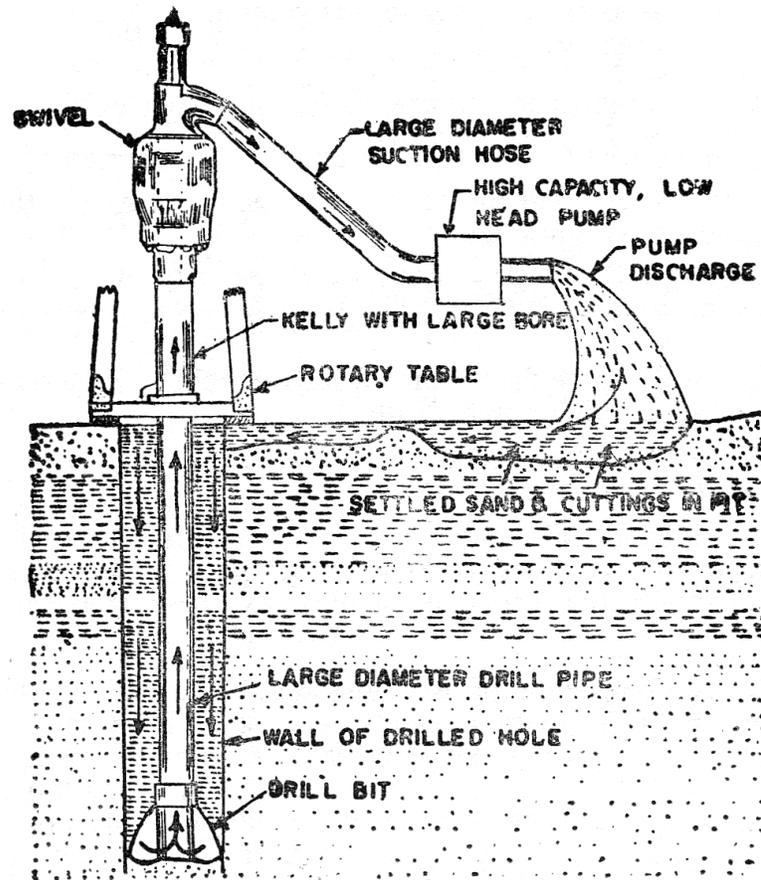
The hole is driven by pumping water under pressure through the drill bit, while it is churned up and down.
