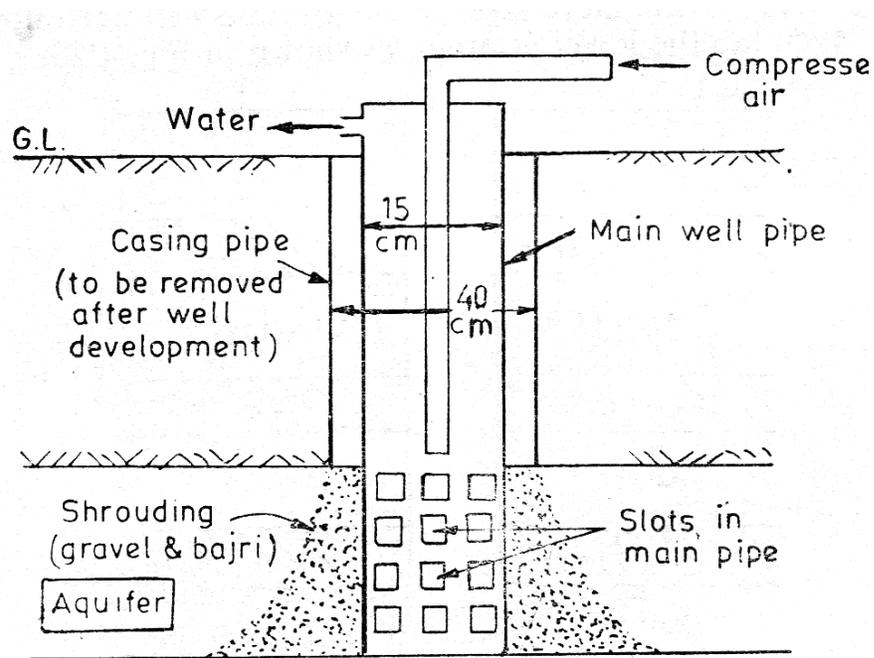
particles into the pipe, the pipe is surrounded by a mixture of gravel and bajri. This mixture is called shrouding and is poured from the top into the annular space between the strainer and
