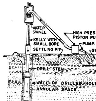
table which fits closely around the Kelley, and allows the drill rod to slide down, as the hole progresses.
