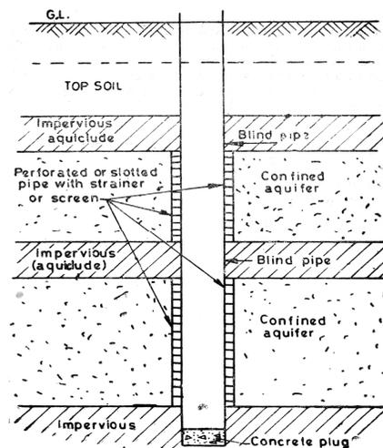
The boring for such a well is generally carried out by a "casing pipe of about 5 to 10 cm larger than the diameter of the well pipe. Thus, for a 15 cm diameter well, a bore hole of 20 to 25 cm diameter shall be drilled. After boring the hole, the well pipe assembly which is partly in ordinary plain pipe (called blind pipe) and partly of strainer pipe, is lowered into the
