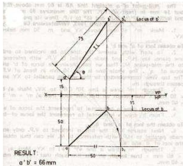
1. Point A is 15mm above HP and 50mm in front of VP, mark  $a'$  15 mm above XY and a 50 mm below XY on the same projector.
