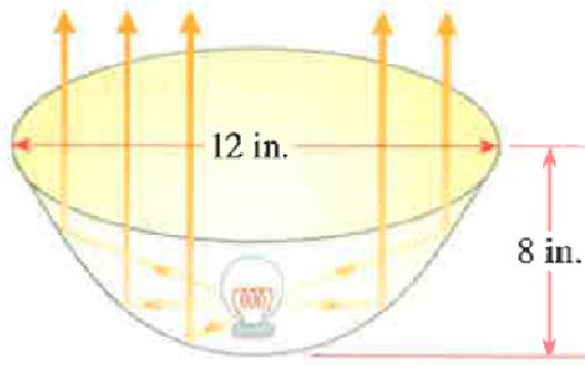
(a) Parabolic reflector
