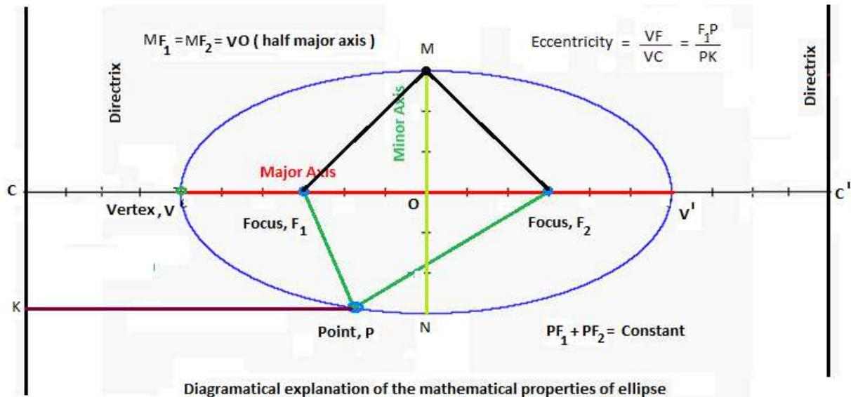
**From each point on the curve, the distance to the focus equals the distance to the "directrix"**
